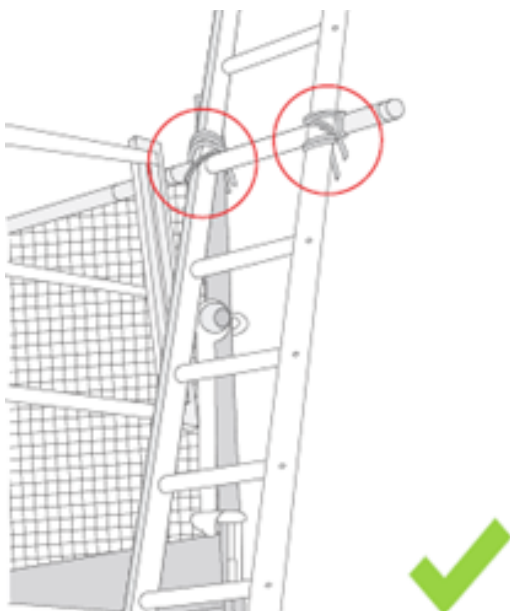
(Fig. 2) vertical access ladder with both stiles tied.
